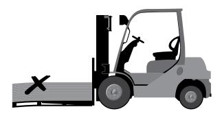
Ensure you use the right forklift length for the laminate stacking height and sheet size. Don't overload the forklift.
